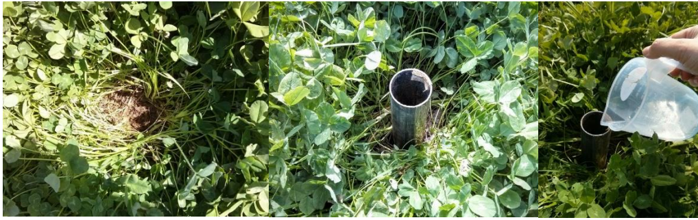
Figures 17-19: Simple infiltration rates measurement.
