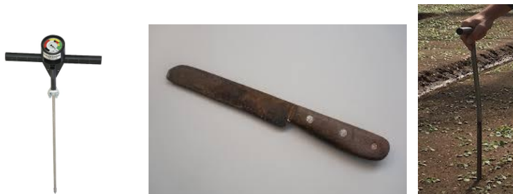
Figures 20 and 21: Penetrometer and simple compaction tools such as blunt knife or soil corer.
